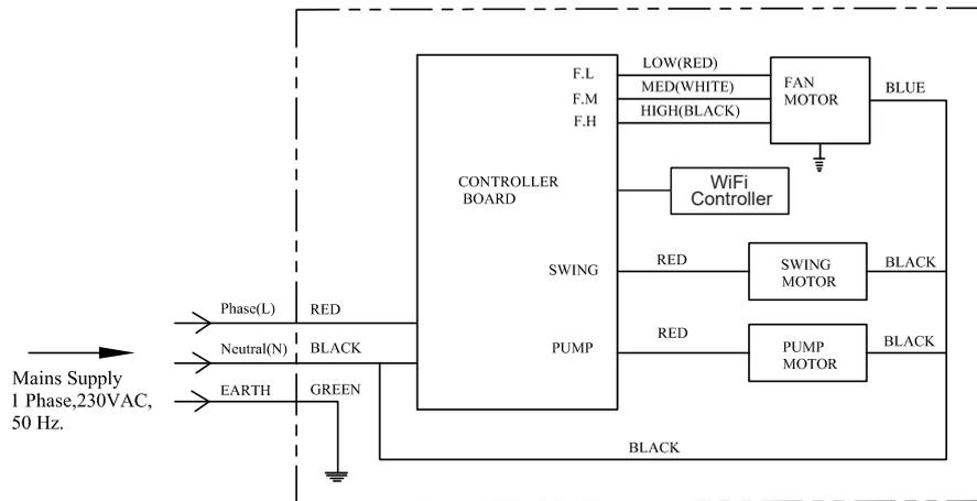
Air Cooler Wiring Diagram ( Wi-Fi Model )
