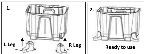
1. Unpack the packing box and take out the cooler along with 2 legs
