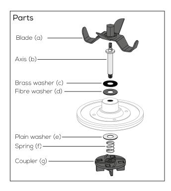
2. If the coupler is removed (the blade sticks together with the axis), washer sand spring will come off when you take blade assembly out of the jar.
